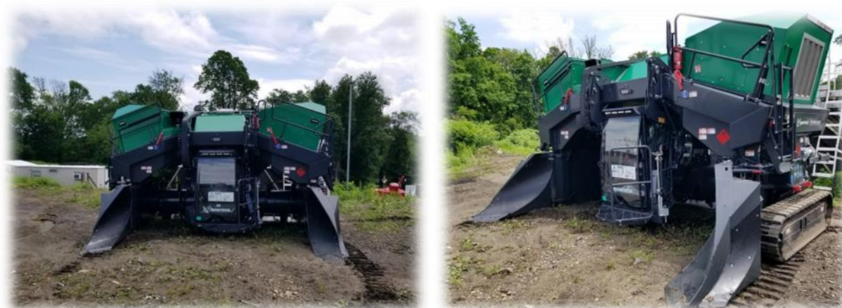
Front and Side Profile of the New Komptech Americas Topturn X5000 Windrow Turner at the MCMUA Mount Olive Vegetative Waste Recycling Facility
